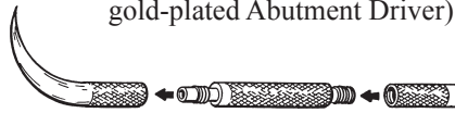
Locator Core Tool No. 8393 (Male Removal Tool, Male Seating Tool, & gold-plated Abutment Driver)
